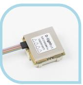
Directly compatible with most digital balanced signal protocols, the 10+ G range meets IEEE std 10G Base-SR10, Fiber Channel, Infiniband, SFPDP, sRIO and VSR requirements as well as ARINC 818 and DVI video standards.
