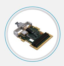
Expand the I/O capabilities of your FPGA board with high-speed and high-density optical links without re-design. The TechwaY WildcatFMC board provides all the benefits of D-Lightsys® transceivers on a VITA FMC compliant plug-in device.
