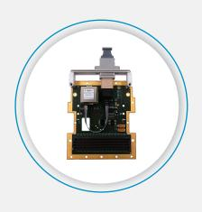
Scalability of signal processing electronic systems is a key point to keep benefits from last state-of-the-art technologies, in particular the latest high-speed I/O capabilites of the FPGAs. WildcatFMC provides system designer with a plug-in solution handling high speed multichannel optical I/O interface for demanding applications.
