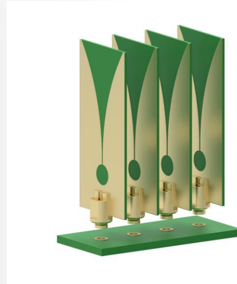
IMP-LP encapsulated in an edge receptacle
